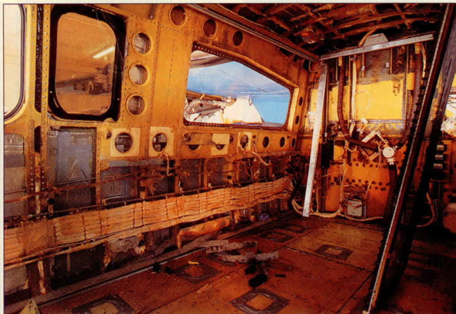
Before: Interiors are ripped out, the entire airframe is inspected, and any problems are corrected. After: This new interior with leather seats and all the trimmings was done by Byerly Aviation of Peoria, Illinois.
